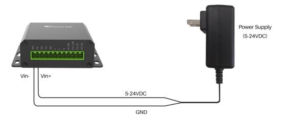
For industrial applications, it is advised that UC1152 should be installed into its own metal housing and be powered from a separate power supply (as opposed to sharing one with other equipment).
