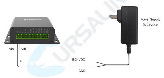
For industrial applications, it is advised that UC3x14 should be installed into its own metal housing and be powered from a separate power supply (as opposed to sharing one with other equipment).
