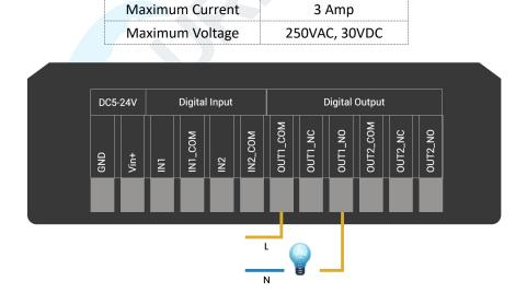
• When the output is off, the COM and N/C terminals will be internally connected to each other. Here is a schematic of the output circuit:
