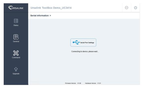
When the Ursalink ToolBox displays: **Connecting to device, please wait...**You can click **Serial Port Settings** to set the correct serial port parameters.
