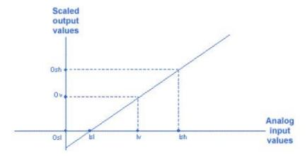
The following formula for calculating the scaled value can be derived from the diagram:
