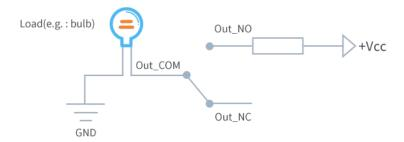
• When the output is on, the COM and N/O terminals will be internally connected to each other. Here is a schematic of the output circuit:
