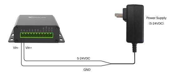
For industrial applications, it is advised that UC3x22 should be installed into its own metal housing and be powered from a separate power supply (as opposed to sharing one with other equipment).
