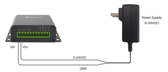
For industrial applications, it is advised that UC3x52 should be installed into its own metal housing and be powered from a separate power supply (as opposed to sharing one with other equipment).
